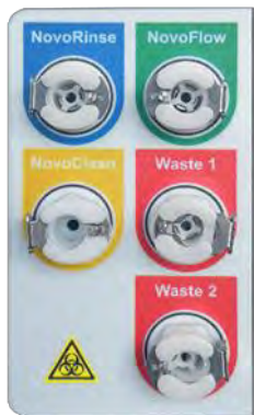
Figure 25. Interface of the Fluidics Ports
