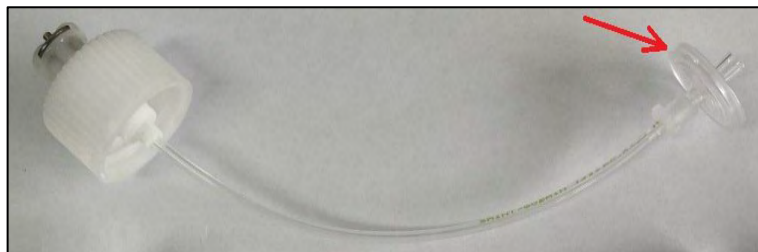
Figure 101. NovoRinse and NovoClean Solution Inlet Filter
