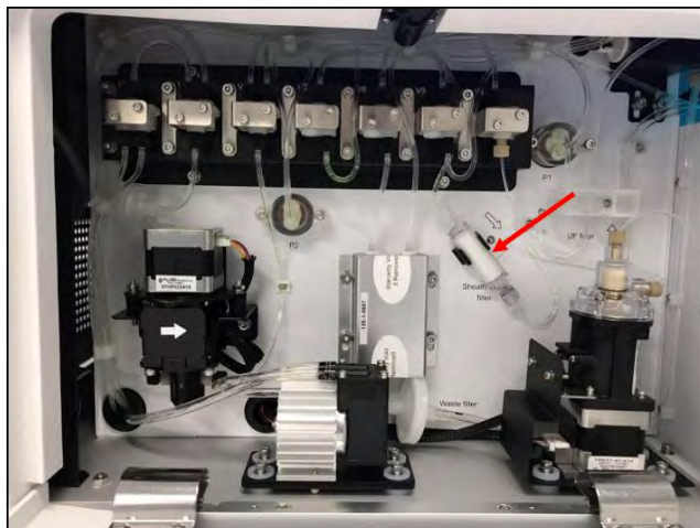
Figure 97. Location of Sheath Fluid In-line Filter
