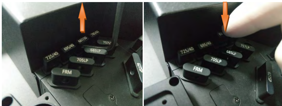
Figure 29. Change the Optical Filter or Dichroic Mirror
