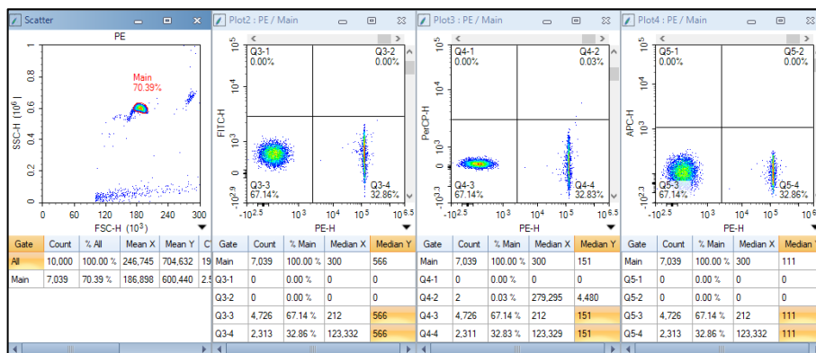
Figure 63. Compensate PE Spillover into FITC, PerCP and APC Channels
