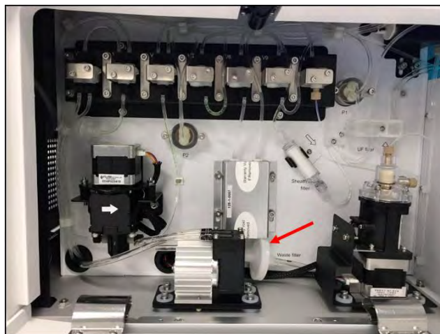
Figure 98. Location of Waste Filter
