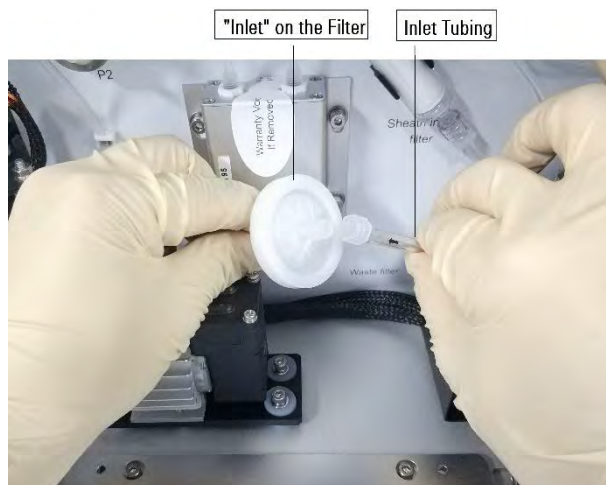
Figure 99. Connect the Waste Filter
