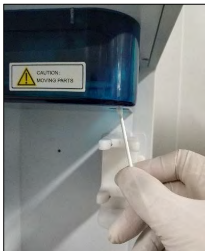
Figure 86. Wipe the SIP Cleaning Apparatus' Lower Surface
